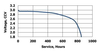
Pulse Drain: 2 seconds X 12 times/day 400 ohms 6.8 mA @2.7V
